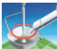
Desoldering IC component with hot air
