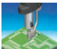
Cleaning pads with desoldering iron
