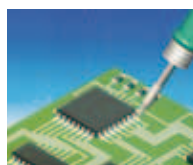
Soldering from 2 opposite angles
