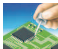
Fluxing IC pads and leads
